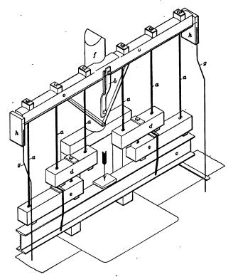
Fig. 46.—Method of testing cross-arms.
